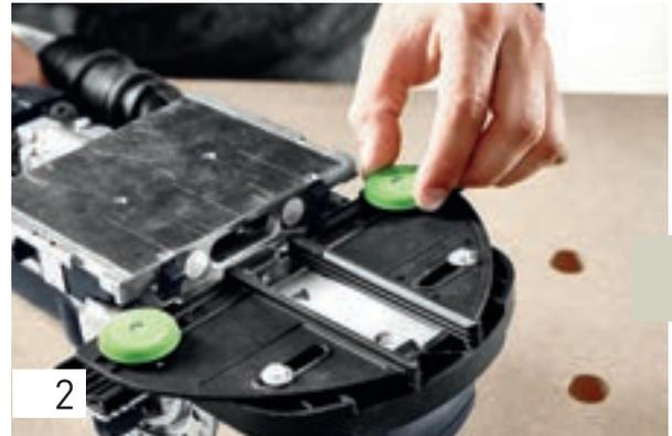
Set the width of the trim stop to the thickness of your spindle by adjusting the guide in the parallel side fence to the correct dimension using the scale and the green rotary wheels. In this example, we are working with 30 x 30 mm rectangular spindles.
