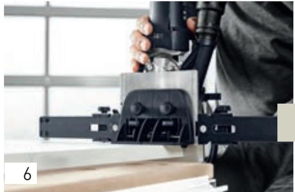
Use the same process to create the routed holes for the side wall of the cabinet. Set the first hole with the stop pin of the DOMINO joining machine...
