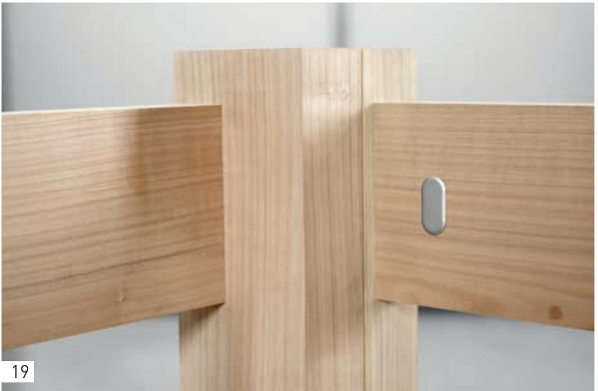
This is a quick way to create a stable joint that can be quickly disassembled if necessary, without time-consuming measuring or marking.
