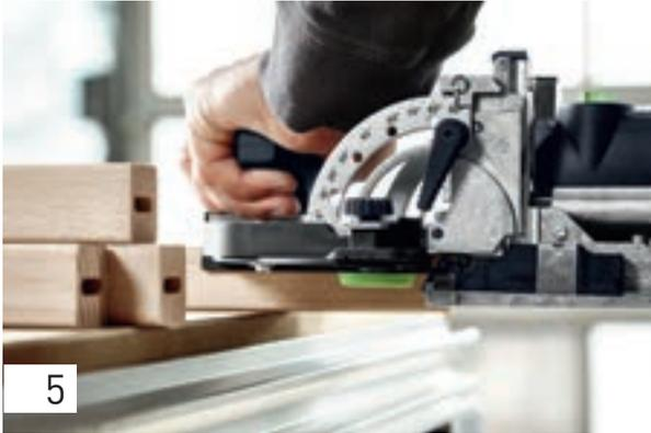
Set the routing height to 15 mm, so that the domino is centred on the spindle later. Set the routing depth to 20 mm, so that the 40 mm domino is later positioned evenly between the spindle and the handrail. Route the hole in the spindles using the narrow hole setting.
