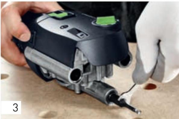
Hold the spindle lock on the motor unit, loosen the cutter using the open ended spanner and screw off. Screw in the new cutter using the open ended spanner, keeping the spindle lock pressed. Then release the spindle lock.
