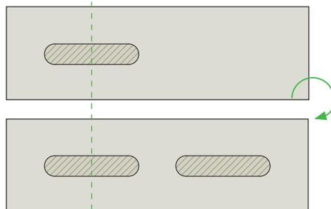
The pins allow two domino holes to be placed by rotating the workpiece, e.g. for the same moulding cross-section.
