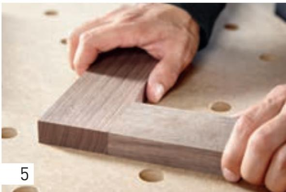
Then glue the frame rail and brace with pads and clamps, if necessary.
