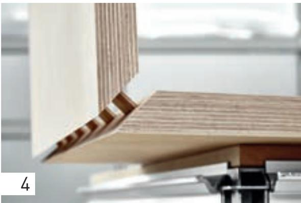
Then join the workpiece parts together, gluing the dominos carefully in the process.
