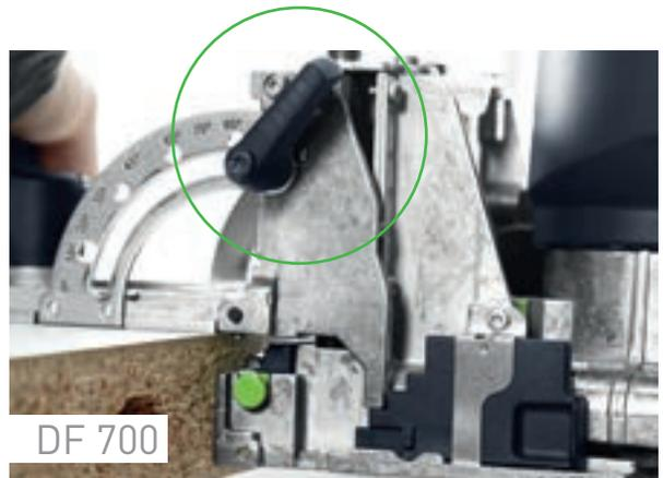
**DF 700** The routing height is adjusted on the DF 700 equivalent to the DF 500. The only difference to note: here, the preselect setting does not determine the board thickness, but instead the true distance from the top of the workpiece to the centre of the routed hole.
