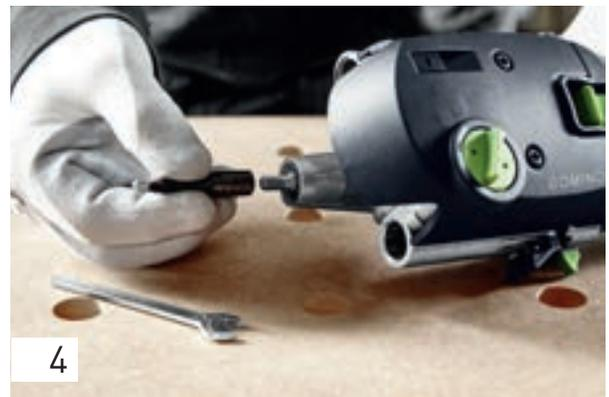
To process a 6 x 40 mm domino as in this example, use the 6 mm router (6 mm dominos can only be processed with the DF 500). For details on changing the router, see chapter 1.4.4, page 18.
