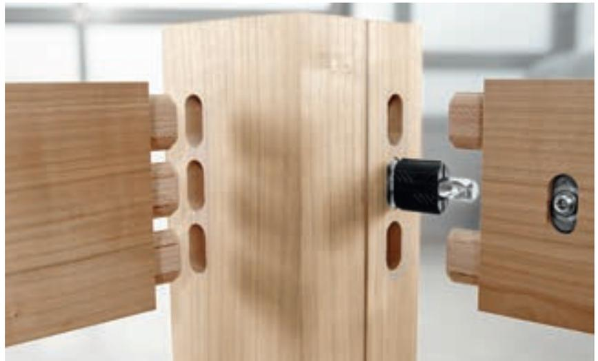
**TIP** It is usually a good idea to fit flexible connectors to one of the sides and securely glue dominos into the other side.
