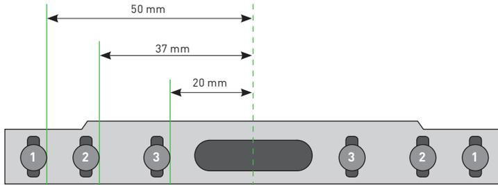
The stop pins serve as distance pieces to the router centre and can be separately located.
