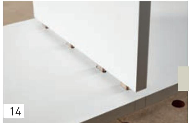
Proceed likewise for the second side part. Then insert the domino in the routed holes and join your workpiece together, applying glue to the joint.
