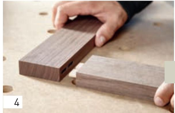
Use this method to carry out routing for all four frame rails, whereby every second frame rail is routed into the workpiece lengthwise instead of into the front.
