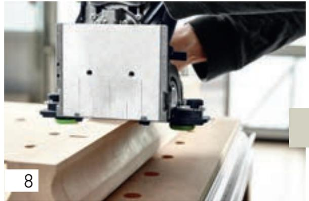
Route the holes in the handrail, positioning the joining machine on the second marking.
