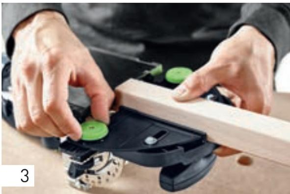
Using the spindle as a guide, ensure that the trim stop dimension fits perfectly; make further adjustments if necessary.
