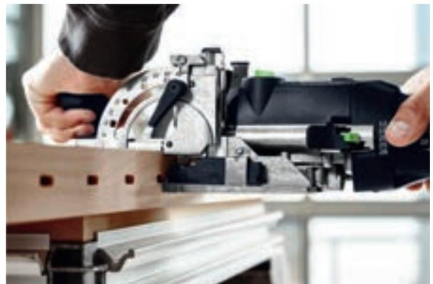
Set the routing height to the centre of the workpiece. Mark out the axis distance of the spindles on the top side of the workpiece. In this case (when simply using markings) bring the scale in the viewing window of the DOMINO over the scribe mark and set the routed holes. A second scribe mark, as in the example of the handrail above, is not necessary here.
