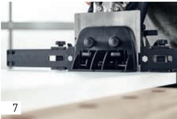
...and create the others using the cross stop pins. Using the additional stop, along with the cross stop – is beneficial here, because the joining machine has a sturdy support surface on the panel.
