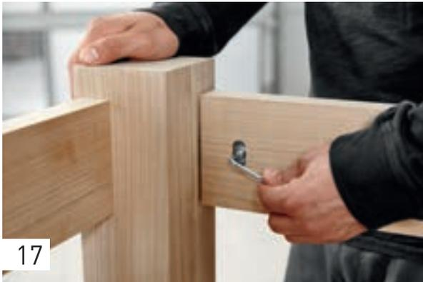
Tighten the connection using a 4 mm hexagonal socket.
