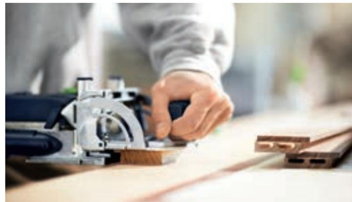
**TIP** If the frame rail needs to be rebated or grooved, the rebating depth must be added in advance when routing the domino holes, so that the domino is centred later despite the rebate (which then takes up part of the depth of the domino hole).
