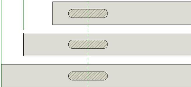
Pins (1 - 2 - 3) allow three separate distances to a reference edge.
