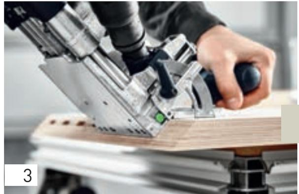
After routing the first hole (the pin is positioned at the edge of the workpiece in this case), the pin goes into the routed hole, thus setting the next stop. Route the first hole with precision, and all other holes as slots with clearance.
