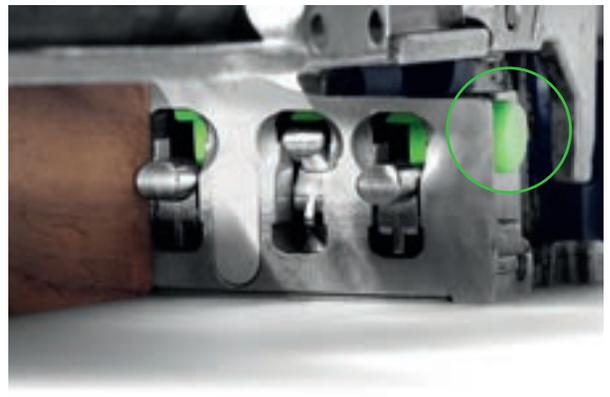
There are six stop pins on the stop side of the joining machine. Unnecessary stop pins can be pushed aside individually and lock in place, and can all be released again by pressing the button on the side of the machine (see markings in the figure).
