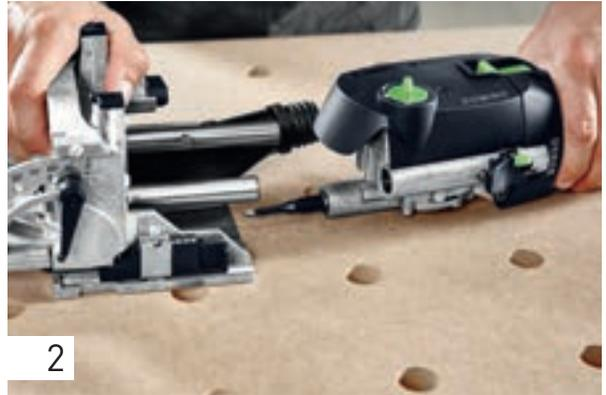
Separate the motor unit and guide frame.
