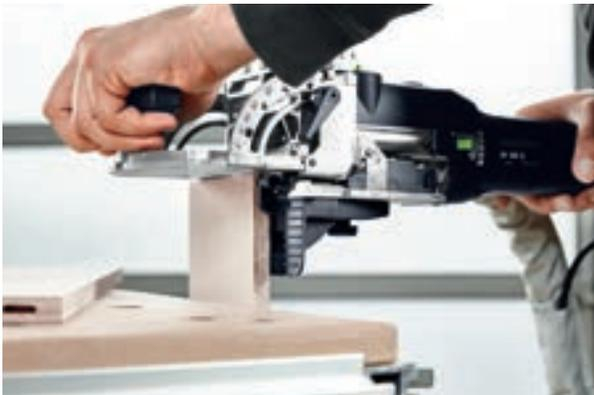
**NOTE** Of course, butted joints are also possible using the smallest domino. Proceed as described above and route the domino holes on the front side using the additional stop.
