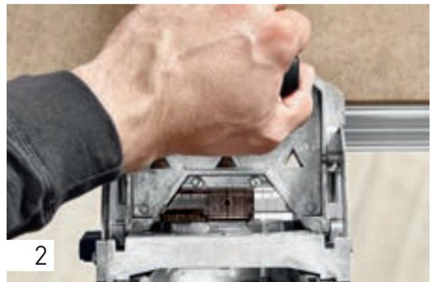
The routed holes can be set by marking them out as usual or using the stop system with the scale in the viewing window – in this example, 15 mm from the outside edge. For this option, place the scale with the 15 mm marking at the edge of the workpiece.
