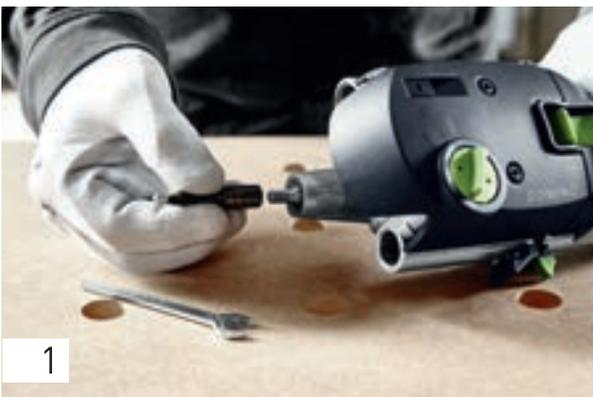
Before starting, ensure that the correct router is used. In this example, we are processing an 8 x 40 mm domino, so the 8 mm router must be used.
