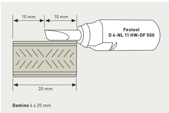
**ATTENTION** The D 4-NL 11 HW-DF 500 specialist cutter is available for the 4 x 20 mm dominos. Please use a routing depth of 20 mm when working with this domino and cutter. However, the true routing depth is 10 mm, because the specialist cutter has been shortened by 10 mm due to the risk of fracture. This domino can only be positioned centrally.
