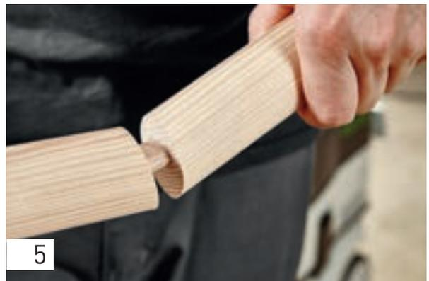
Insert the 8 x 40 mm domino into the routed hole, applying glue to the joint. Then join the two workpiece parts together – the joint is secured from twisting with just one domino!
