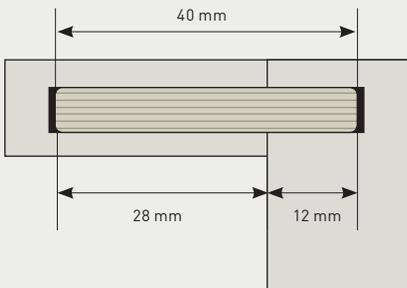
**Example:** The domino being used is 40 mm long; the left hole is 28 mm deep, the right hole 12 mm – that is, together 40 mm.
