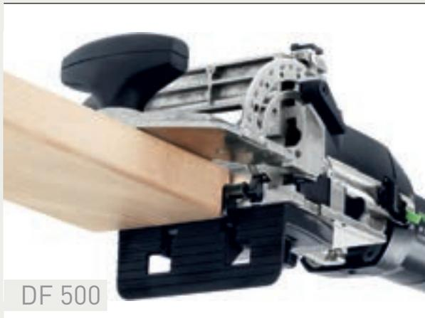
The additional stop provided with the DF 500 increases the contact area and reduces the lateral distance of the stop catches to the DOMINO centre from 37 mm to 20 mm. This allows precise positioning of narrow workpieces.
