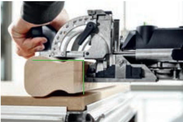
**CAUTION** Especially with handrails, it is often not possible to position the joining machine securely on the side of the workpiece due to the handrail design; the round shape prevents the DOMINO joining machine from having a secure support surface.
