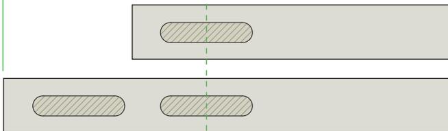
The pins allow two domino holes to be placed adjacent to each other at a defined distance to a reference edge (1 - 3).
