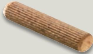
Round dowels are one of the most important connecting elements in furniture making, allowing timber connections to be quickly and reliably aligned. Because round dowels do not allow offsets, exact drilling is generally performed on stationary or semi-stationary machines.
