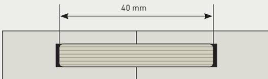
**TIP** The domino should generally be centred within the joint; that is, the routing depth should correspond to half of the domino length. However, depending on the workpiece or joint type, it may be necessary to locate the domino randomly. In this case, both of the holes routed in the workpieces must together correspond to the length of the domino being used.
